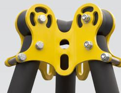
The head is made of powder coated aluminum and has three ball-bearing wheels for guiding the work rope on rescue or lifting devices.
