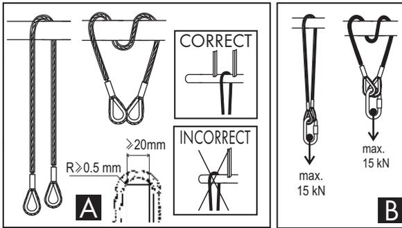
2. The maximum allowable working load of the AZ410 lanyard (used as a temporary anchor point) is 15 kN. The structural anchor point static strength must be at least double of working load of the AZ410 (which is transmitted in service from the AZ410 lanyard to the structure) but not less than 12 kN - drawing B.
