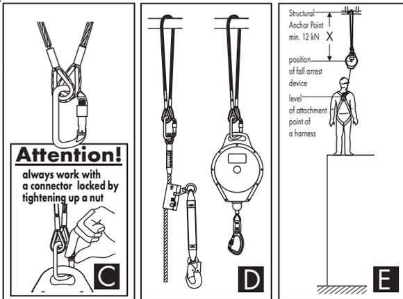
5. Connect a fall arrest device (e.g. retractable type fall arrester, guided type fall arrester, etc.) to the lanyard's snap hook - drawing D.
