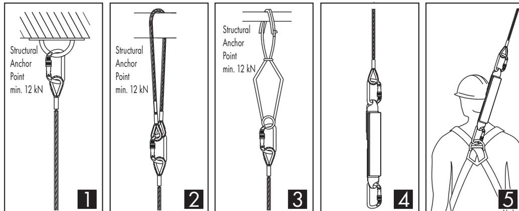
IT IS STRICTLY FORBIDDEN to use tyhe AZ410 lanyard without the energy absorber.as a fall arresting device. The total length of the sub-system with connecting lanyard AZ 410 including an energy absorber, terminations and connectors shall not exceed 2 m.
