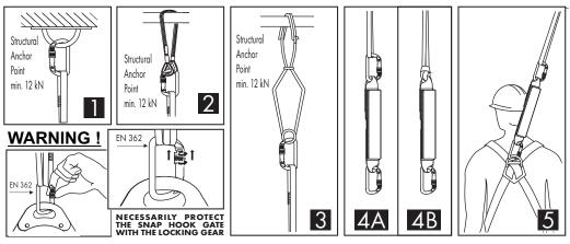
ITES: - In determining the space under the workplace required to arrest the fall, consider the sling as an additional element that extends the distance for arresting a fall.
