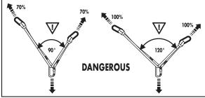
the structural anchor point should be situated above the working place and the shape of the structural anchor point should not let self-acting disconnection of the webbing sling connector.
